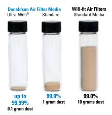
Filtration efficiency (%) and dust passed after exposure to one kilogram of dust (approximately 100 hours of operation) for a typical off-road application.
