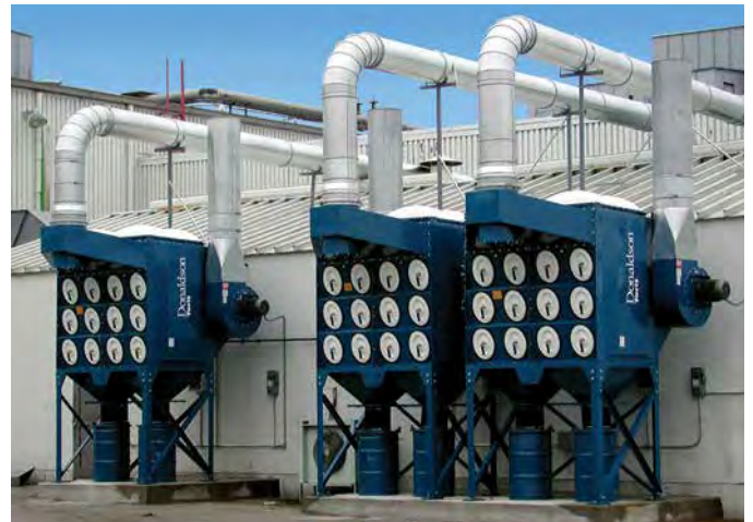
DFO on Metallizing Powder Flame 20,500 cfm (34,822 m 3 /h)
