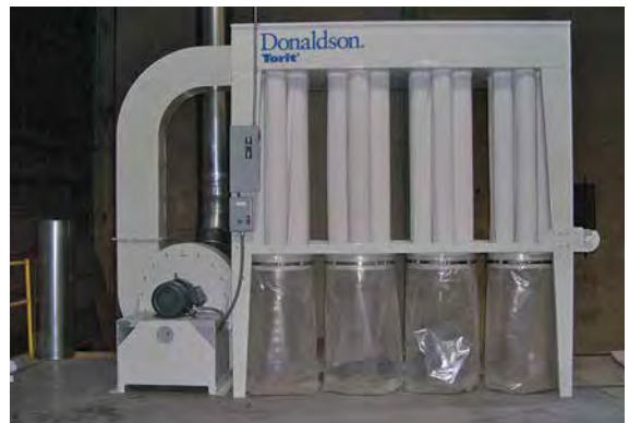
IRD - Wood Shop 5,000 cfm (8,493 m 3 /h)
