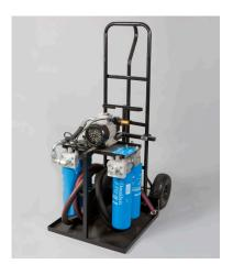
The Donaldson Bu.F.S.S. provides off-line filtration and fuel transfer capability in a convenient portable package.
