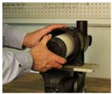
If you perform filter maintenance service on a schedule versus using service indicators, you may want to write the service date on the end cap of both filters.
