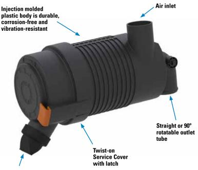
45° Vacuator™ Valve orientation permits either vertical or horizontal air cleaner mounting (the dust cup can be incrementally rotated to suit specific applications)
