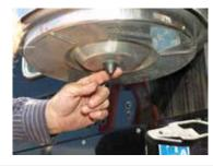
**Inspect the Old Filter** Inspect the old filter for any signs of leaks. A streak of dust on the clean side of the filter is a telltale sign. Eliminate any source of air leaks before installing the new primary filter.
