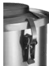
ECG style air cleaners have three cover latches that need to perform correctly to ensure the filter gasket is sealing properly. These latches should be checked for tightness and wear. To check
