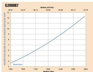
\*\*Results generated using laboratory testing pursuant to ISO5011. Actual performance during use may vary depending on multiple factors, including specific product configuration, external conditions and application.
