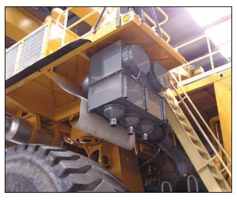
The large, massive mining vehicle in the picture above is an ideal match for the Donaldson SSG Air Cleaner.
