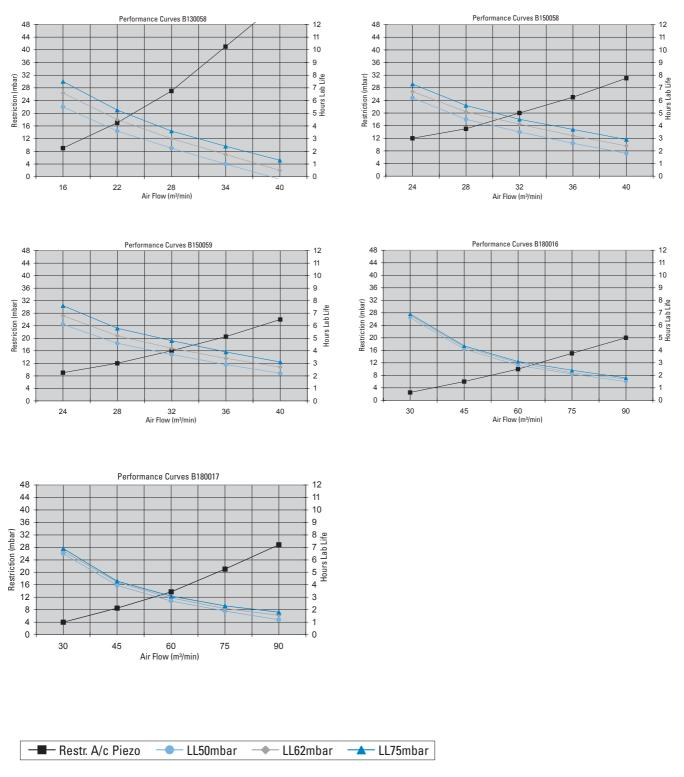
All performance curves are according ISO 5011 standards - Restriction measured at Piezo All tests are done with ISO Coarse at Dust Concentration of  $1g/m^3$
