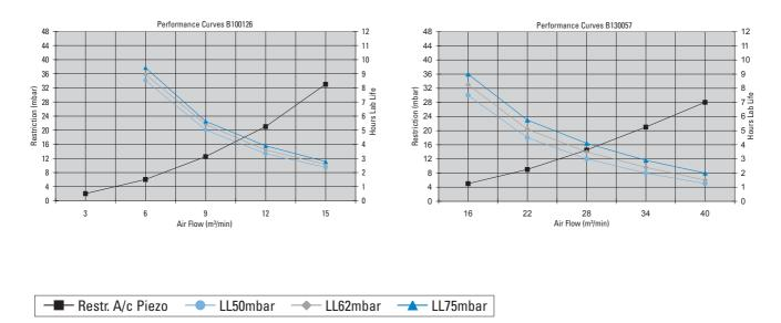
All performance curves are according ISO 5011 standards - Restriction measured at Piezo All tests are done with ISO Coarse at Dust Concentration of 1g/m<sup>3</sup>
