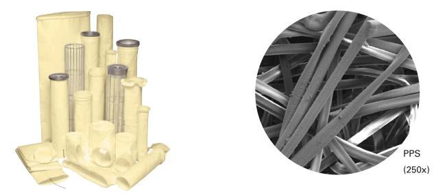
Needled 16 oz. PPS (polyphenylene sulfide) felt is a high temperature filtration media used in pulse jet baghouse dust collectors. This material performs well in applications where alkaline and or chemical resistance is required. It also works well in applications with moisture content and where dew point crossings are common. It is strong, abrasion resistant with high resistance to alkalies and acids and good for applications up to 375° F.
