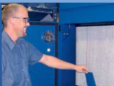
One pivot lever securely retains the primary filter element
