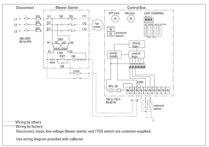
Solid-State Timer Typical Wiring Diagram
