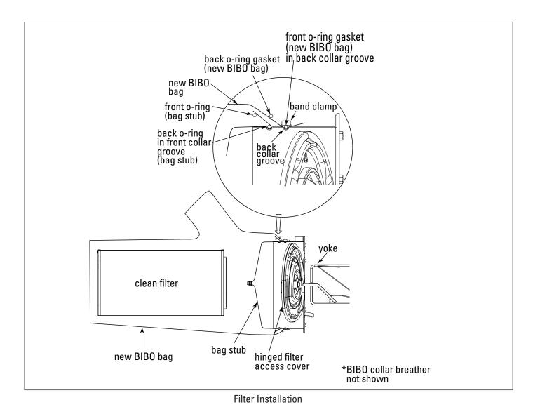
10. Install the filter with gasket end toward collector.
