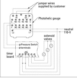
Photohelic Gauge Wiring Diagram
