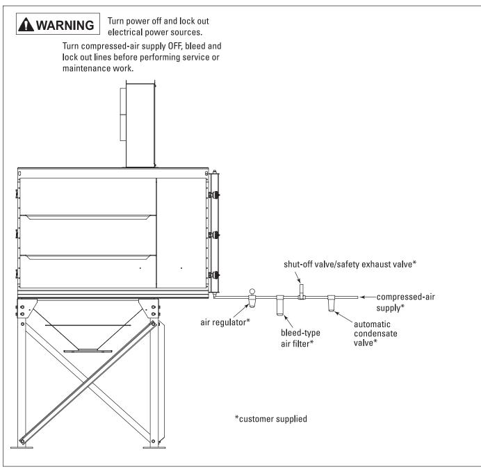
Compressed Air and Component Installation
