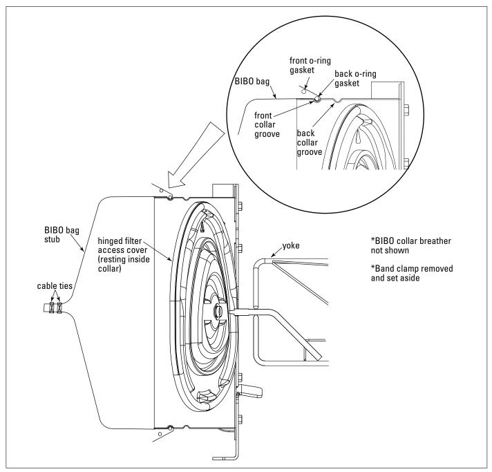
Bag Stub Repositioning (Side View)
