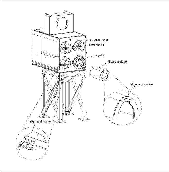
Filter Removal and Installation
