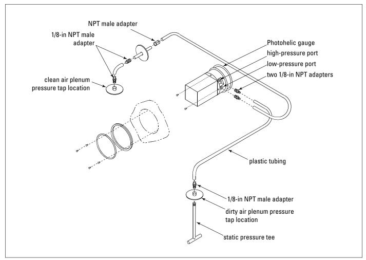
Photohelic Gauge, Remote Panel or Door Installation
