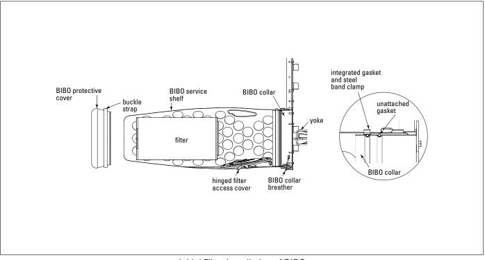
Initial Filter Installation of BIBO
