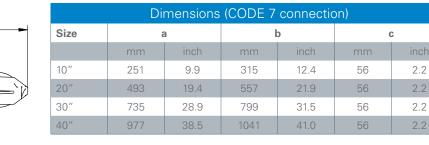
CODE 7:  $2 \times 226$  o-rings, bayonet 2 locking tabs, locating fin, integrated reinforcement ring
