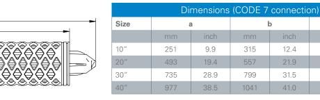
CODE 7: 2 x 226 o-rings, bayonet 2 locking tabs, locating fin, integrated reinforcement ring
